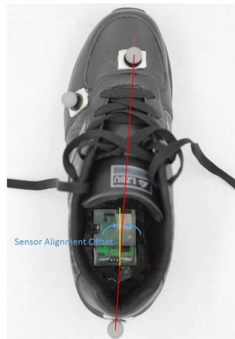
Fig. 3. Sensor alignment offset computed before testing as the angle between the forward horizontal axis of the sensor and a straight line between a marker placed over the head of the second metatarsal and a marker placed over the calcaneus (Shull et al., 2013b).
