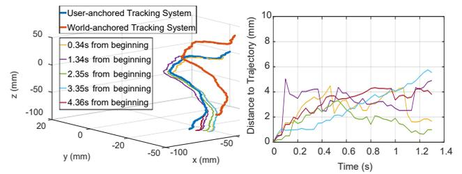
(a) Trajectories of applying static error compensation to the world-anchored within 1.2 seconds (b) Distance to the desired trajectory for compensation to the world-anchored within 1.2 seconds
