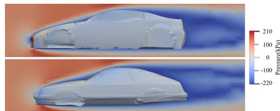
Figure 9. Pressure field before(top) and after(bottom) physics parameters fitting. Drag coefficient of the car on the top is 0.258, on the bottom is 0.203.
