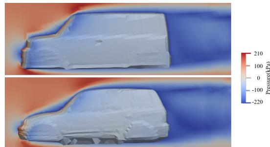
Figure 8. Pressure field before(top) and after(bottom) physics parameters fitting. Drag coefficient of the car on the top is 0.418, on the bottom is 0.348.
